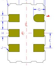
Contacts: Gold 11.8 to 39.4 μinches (0.3 to 1.0μm) over Nickel 50 to 350 μinches (1.27 to 8.89 μm) <sup>1</sup> Typical dimensions
